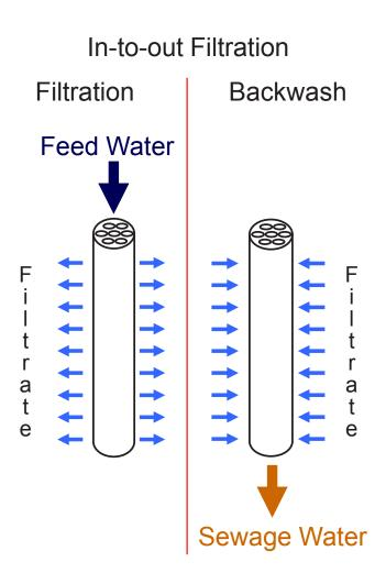
Ultrafiltration is a physical barrier stopping all particles and microorganisms within a limit of 0.02 microns.
